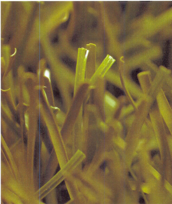
Soccer 65 – Revite ® Brush, 180 cycles. Note split.
