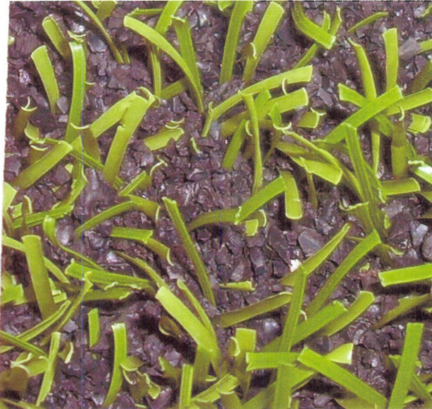
Soccer 65 – Regular Soft Brush – 500 cycles. Note break in fibre top left
