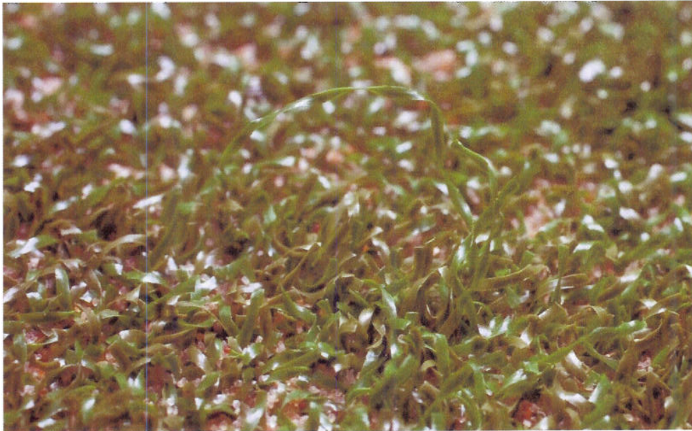
Evolution – Regular hard brush – 10 cycles. Note fibre pulling out.
