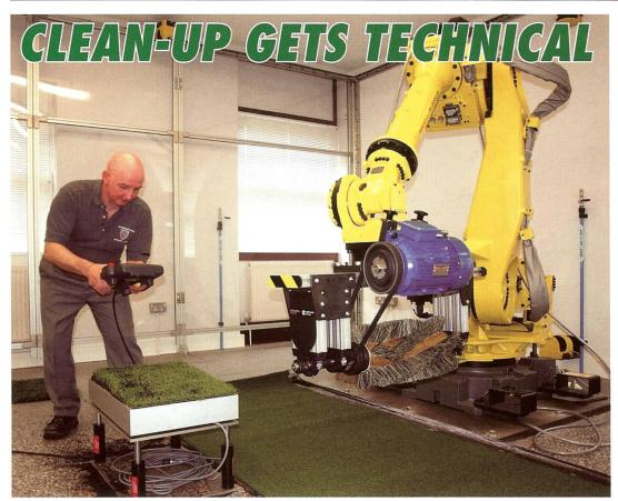
In a unique project commissioned by Technical Surfaces Ltd, Loughborough University's Sports Research Laboratory is using an industrial robot to evaluate various cleaning brushes and their effect on a range of synthetic surfaces.
