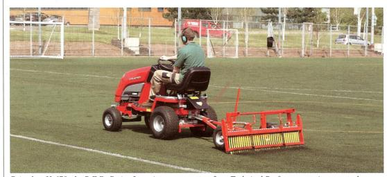
Priced at £3,670, the R.E.D. Series 3x maintenance system from Technical Surfaces comprises a petrolengined power unit with trailed drag mat and Flexicomb attachments. The latter, shown here, has height-adjustable bristles able to drag brush and decompact synthetic surfaces.
